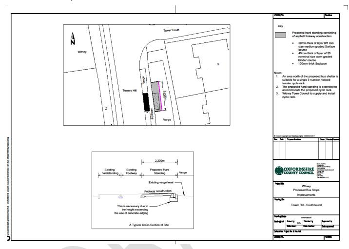
The proposed bus stop shelter is to be installed at the back of the footway in order not to conflict with the existing footway network in the locality.
